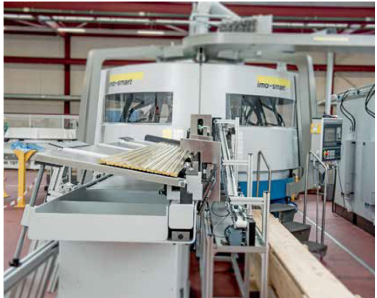
Modularly designed rotary transfer machines from Imoberdorf AG are generally specifically designed according to the requirements of the application.
